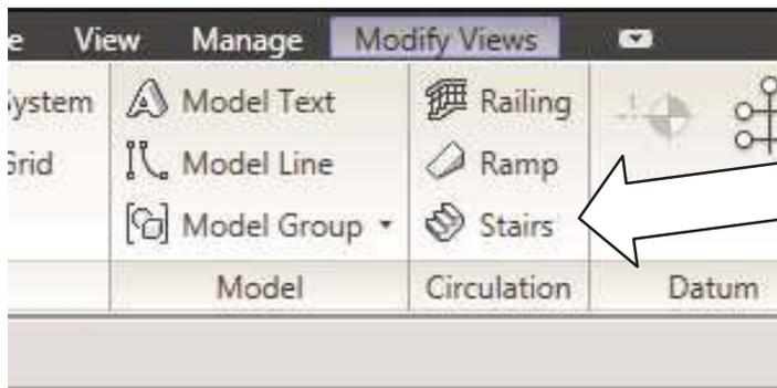
Pick two points to show the direction and length of the stair: pick the first point at a location to the right of the first interior wall. Then move the cursor far to the right and pick the second point. Your stair "sketch" will look like this:
