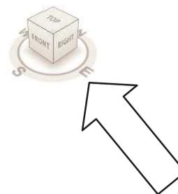
The symbol in the upper right corner of the screen is called the “view cube” where the arrow is pointing toward. This is a sweetie of a tool because it will allow you to navigate to different views of the 3d object. Remember in Revit, you are drawing in 3d all the time. The view cube appears whenever you are in a 3d view.
