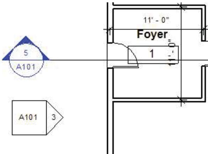
Note that the number of the section and elevation detail on the sheet has been assigned, as well as the number of the sheet on which they appear. If you move the section to another sheet, for instance, the sheet number on the tag will be automatically changed. Revit will not allow you to place a view on more than one sheet.
