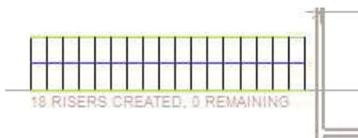
It says “18 RISERS CREATED, 0 REMAINING.” This is a straightforward way of making the stairs, but you can be fancier about it by picking a series of points while “sketching” to allow you to turn the direction of the stairs or create landings. A little practice is warranted to control the sketch creation.
