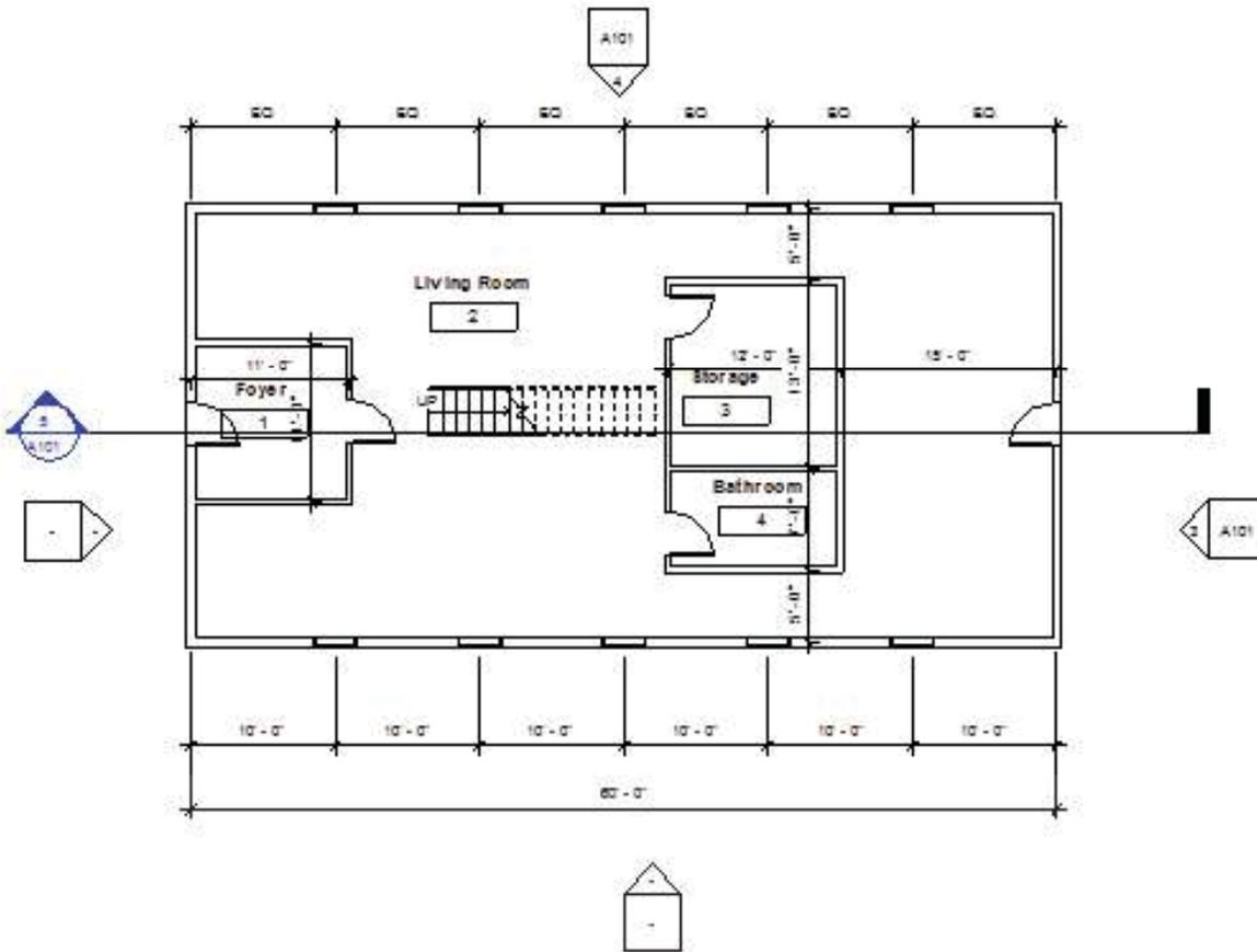
Elevation keys on the Level 2 plan will automatically be moved to the same locations as on the Level 1 plan.
