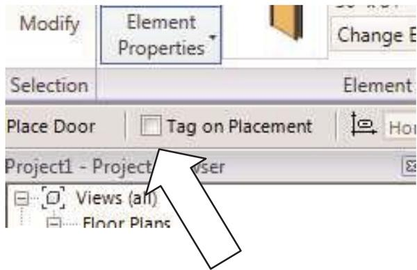
This will not put a door “tag” symbol in the door opening. Door tags are used to reference a door schedule, which we will create later on. To keep things simple, we will just put the doors in for now and add the tags later.
