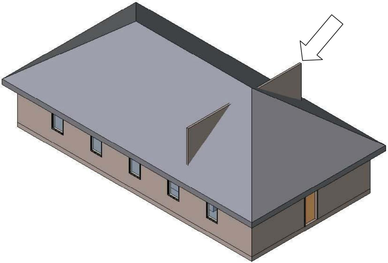
To fix this, click on the wall, and select “Attach” tool on the Ribbon, then pick the roof to attach them to.
