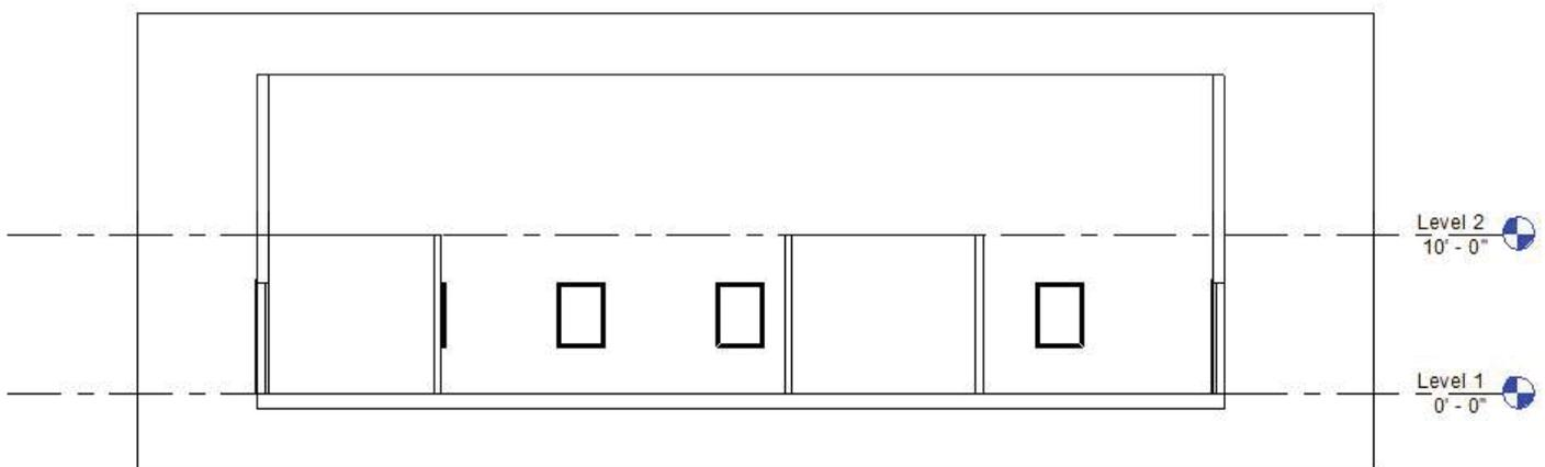
You can clearly see the floor you just created, as well as the level symbols and the interior walls. The outer rectangle around the section itself is called a "viewport" in Revit. It can be adjusted by clicking on it and moving one of the arrows that appears. Let's try it:
