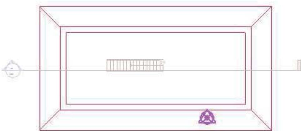
To turn hidden objects back on, right click on the purple object that is visible when the light bulb is turned on and select “Unhide in View”> “Elements.” Then turn the light bulb off.
