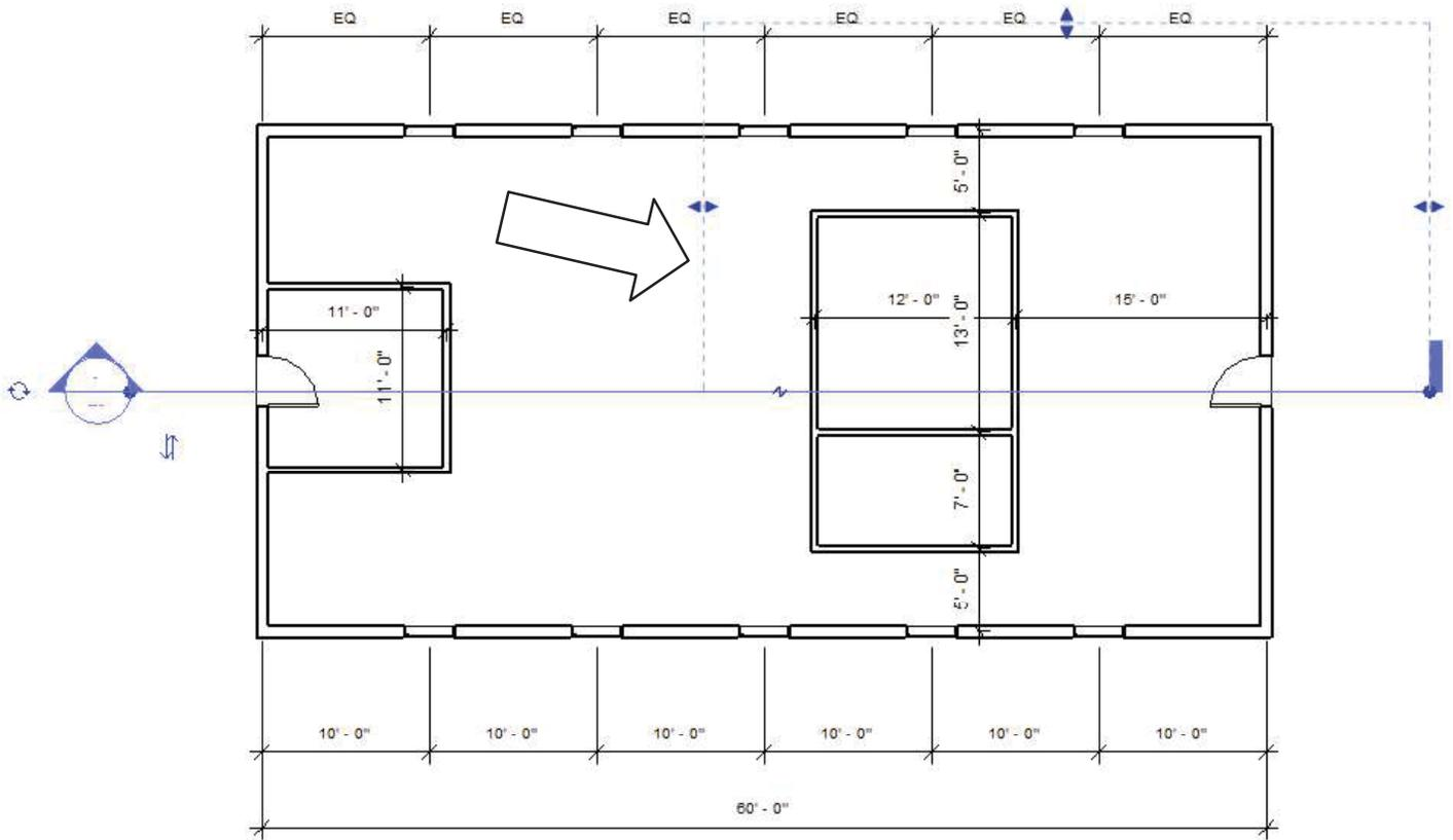
The blue dashed rectangular area above the section line has been shortened to coincide with the viewport area that you changed in section. So there are two ways of limiting the length of the sectional view: change the viewport in section, or change the dashed lines associated with the section mark in plan.
