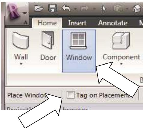
Be sure to uncheck "Tag on Placement" again, just like you did for the doors. Hover the cursor near the point you want to place the window and pick the left button of the mouse. Hover the cursor toward the outside edge of the wall, not the inside edge. If a window gets installed on the inside rather than the outside of the wall, you can easily correct it by clicking on it and clicking on the arrows so the arrows are showing on the outside of the wall.
