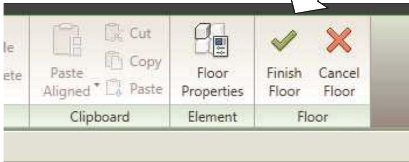
You will get a dialogue box asking you if you want the walls that are below this floor to attach to the bottom of the new floor. Select “Yes.” What that will do is stop the tops of the wall below the floor thickness, no matter how thick the floor will be. If you answer No to this dialogue, the floors will remain attached to the Level 2 plane and thus penetrate through the floor.
