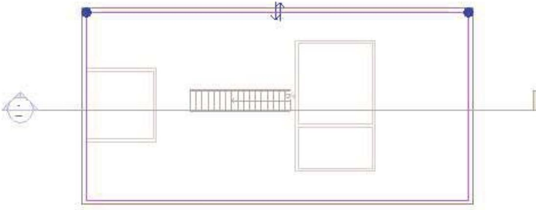
Now we need to cut a hole for the stairs to come through the floor. To do this, select the rectangle on the Ribbon:
