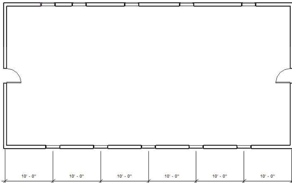
You do not have to do this, but as an example of the equality constraint in action, if I move the right wall 8'-0" to the right, thus lengthening the building, dimensions between all of the windows will change from 10'-0" to 11'-4" maintaining the equality spacing between windows.
