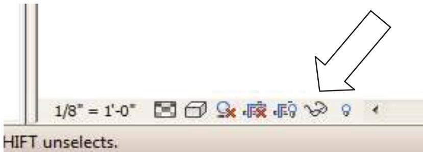
There is an icon on this bar that looks like a pair of glasses. To turn off any object in the view you are in, first select the object and then click on the glasses and pick "Hide Element. "
