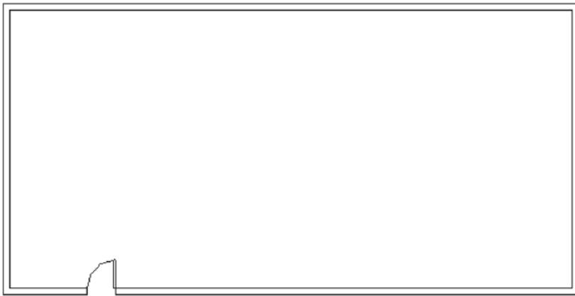
The door may be the wrong size and may be in the wrong location, but that is easy to fix later. You can move the door anywhere along the wall in which it was inserted and you can change both the swing and the hand of the door. Let's practice moving the door along the wall. Select the door. Temporary dimensions will appear:
