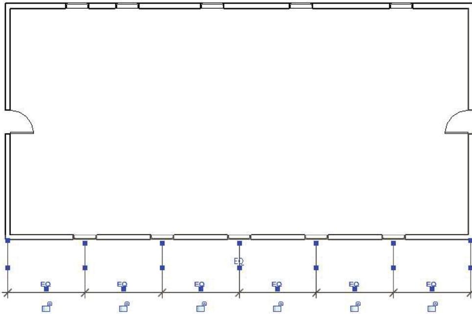
All windows will now move over to be equally spaced and the windows will be “constrained” to this equality spacing regardless of whether the building is lengthened or shortened.
