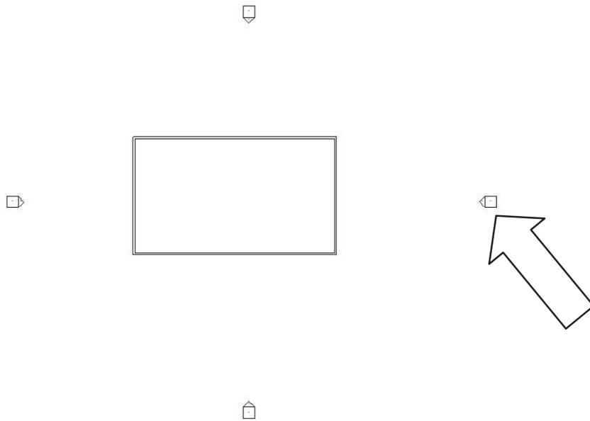
Note that the “home plate” trapezoidal shaped objects are Revit’s (unusual) version of an elevation key (where the arrow is pointing). Revit always starts out drawing a building with two “levels” (floors), although you can change the number of floors by adding more levels.
