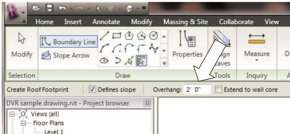
Hover the cursor over the exterior face of one of the walls and hit the Tab key to select all the walls, then click the left button of the mouse. You will get a purple line drawn around the walls 2'-0" away from the walls (this will be the roof overhang):
