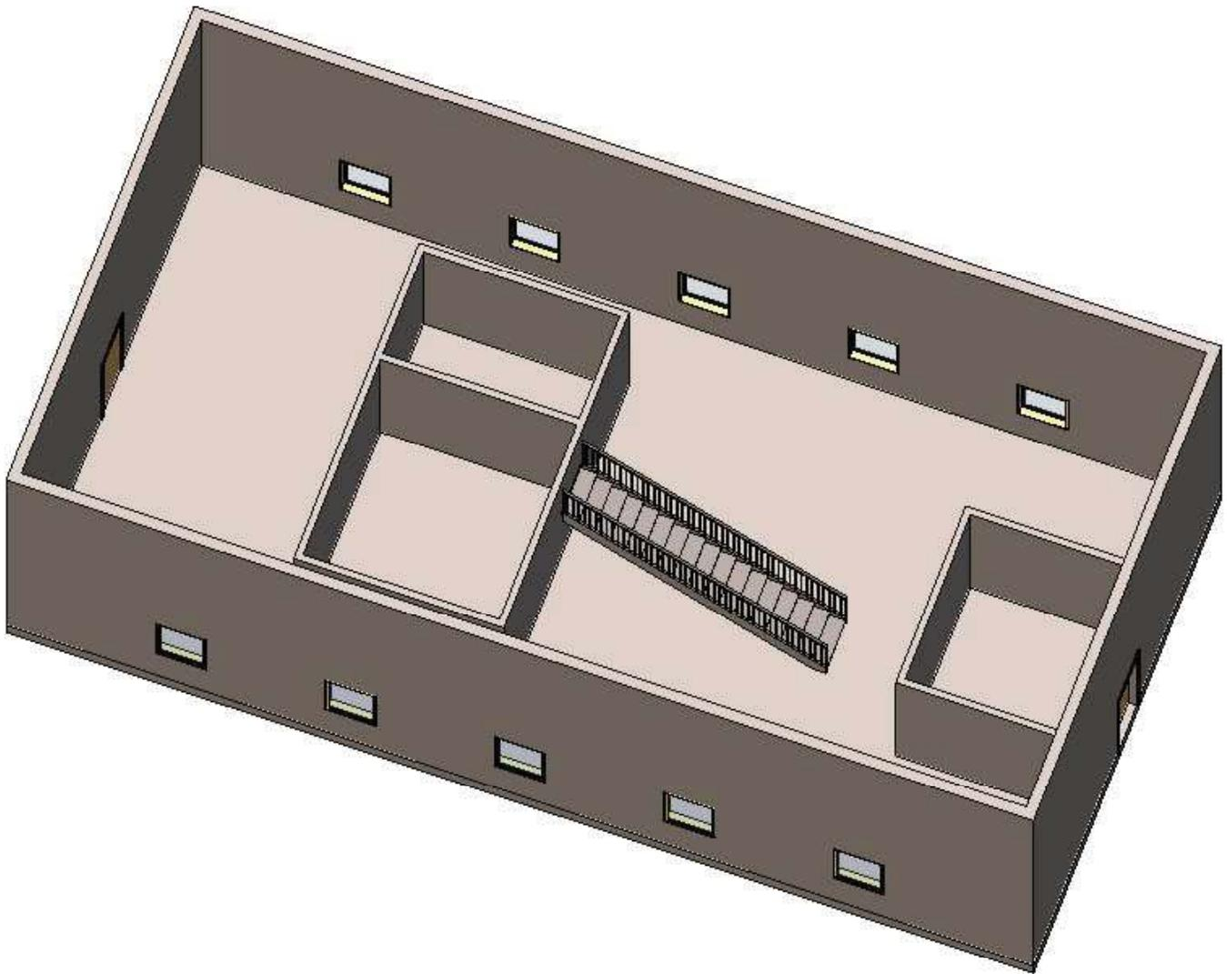
I turned the Shading with Edges on to get it to look like this. The stair by default has railings attached. These are separate objects and can be deleted or changed to a different type if you wish.
