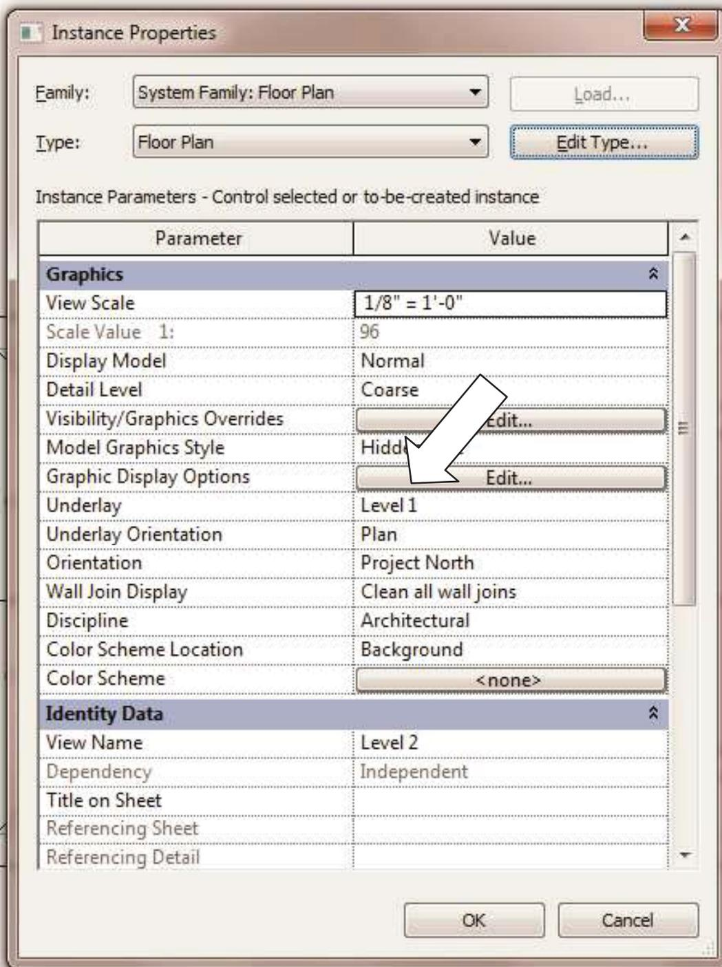
Note that in the “Underlay” row, the words “Level 1” appear. That means that the underlay drawing is Level 1 Plan. You can turn it off by selecting the words Level 1 and a drop-down menu appears giving you a choice of various plans to show as an underlay, including one called “None.” Select “None” and then see that the walls on the first floor are no longer showing as faded out lines on the second floor.
