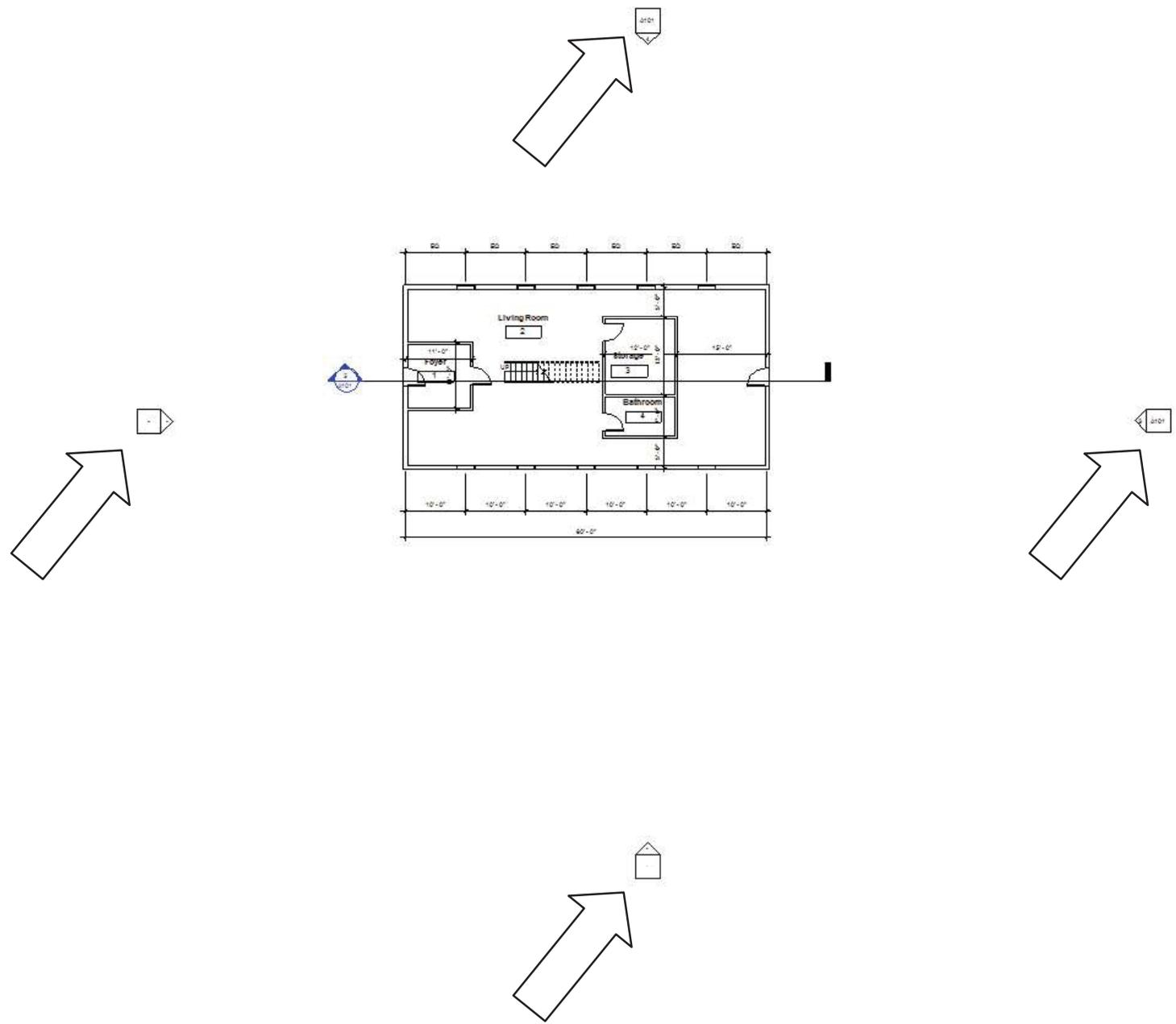
To move an elevation key on a plan, first put a window around the whole key and select the “Move” tool.
