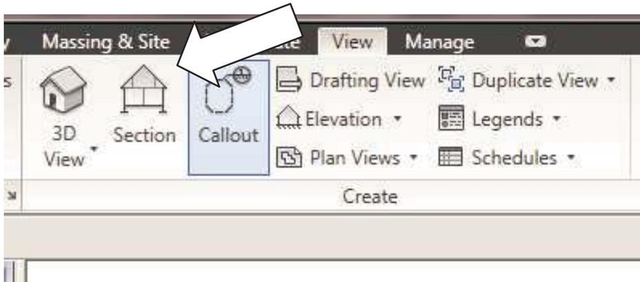
Then pick the Section tool. A cross-shaped cursor will appear. Pick a point on the left side of the plan outside the exterior wall, then a point to the right side of that point, like this:
