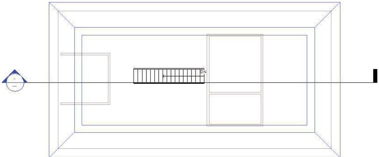
It is an odd appearance, I must admit, but totally rational, because the plan view is cut 4'-0" above the floor level. If you go to the section view, it will look like this:
