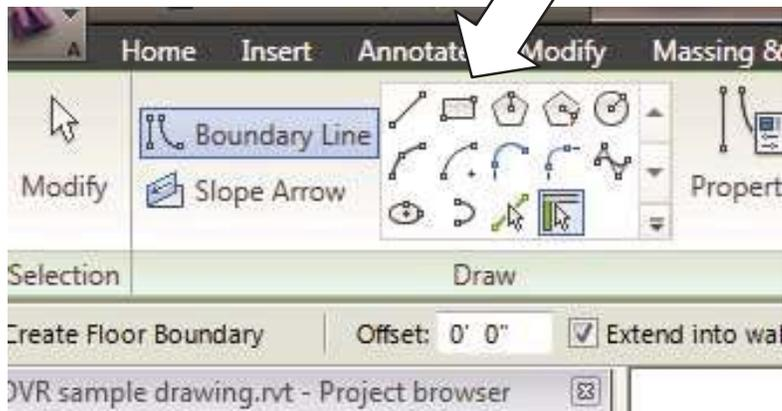
Draw a rectangle around the stairs to make a hole in the slab.
