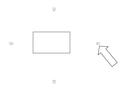
Note that the "home plate" trapezoidal shaped objects are Revit's (unusual) version of an elevation key (where the arrow is pointing). Revit always starts out drawing a building with two "levels" (floors), although you can change the number of floors by adding more levels.
