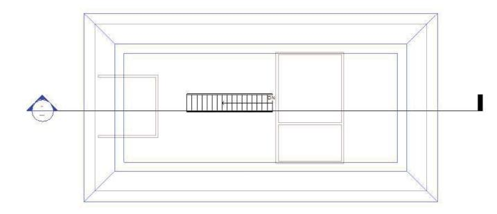
It is an odd appearance, I must admit, but totally rational, because the plan view is cut 4'-0" above the floor level. If you go to the section view, it will look like this:
