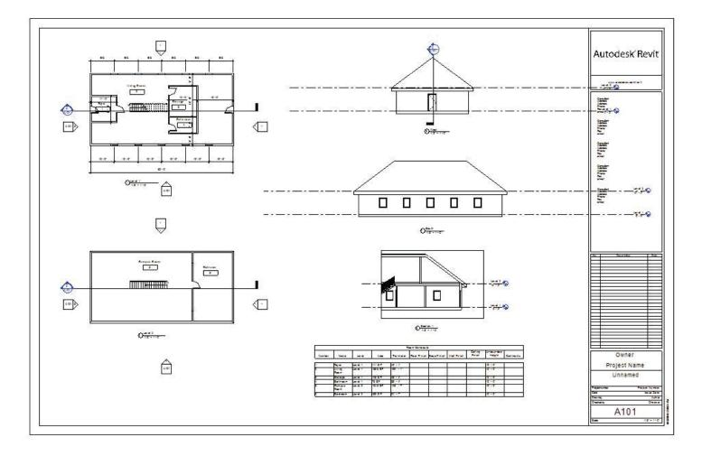
Note that you can create as many sheets as you want using the same process. Every drawing view put on the sheet will be given a number automatically and the tags for Elevations and sections will be shown on the sheet: Zoom in to one of the title numbers:
