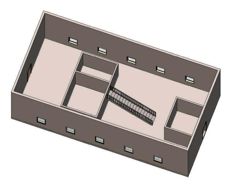
I turned the Shading with Edges on to get it to look like this. The stair by default has railings attached. These are separate objects and can be deleted or changed to a different type if you wish.
