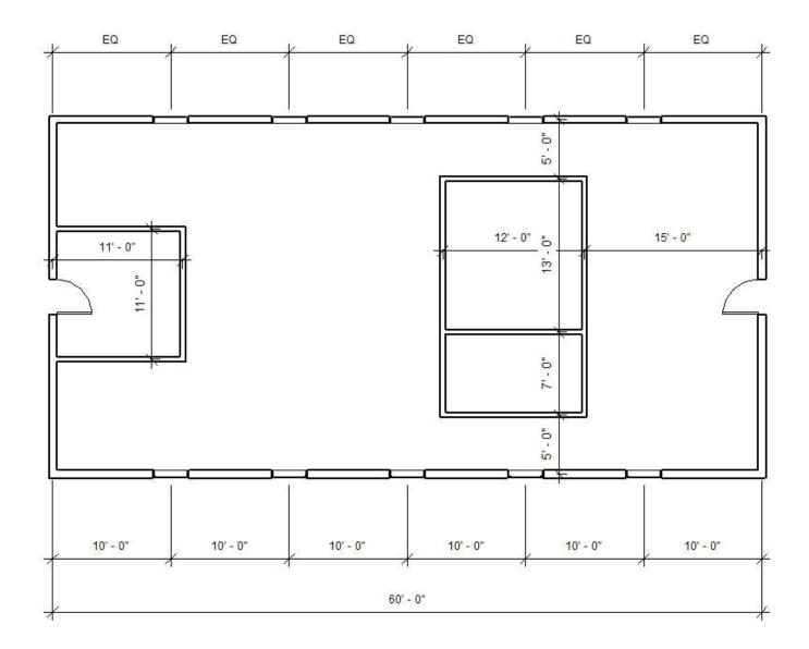
21. Let's put a floor under the first floor. Select the Home tab and select the "Floor" tool. The drawing will dim and the instruction at the bottom of the screen will now say "Pick walls to create lines." Hover the cursor above the outside edge of the top wall and then hit the TAB key on the keyboard; immediately click the left mouse button. A purple line will appear all around the outside of the exterior walls. You may need your instructor to show you how to do this properly. Be patient.
