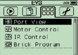
Now you can use port view to get the exact real-time readings of your connected sensors.
